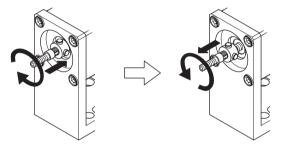
3. Insert the ball screw shaft into the installation hole for the shaft on the flexible plate and then fix with the nut. (Fix with a screw for  $DR\square42$  or  $DR\square60$ .)
