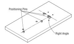
2. Pressing the reference surface of the guide rail against the positioning pins, fix it with screws.
