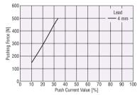
The characteristic diagrams above show the averages of measurement results of pushing during horizontal operation of the DRS2 Series.
