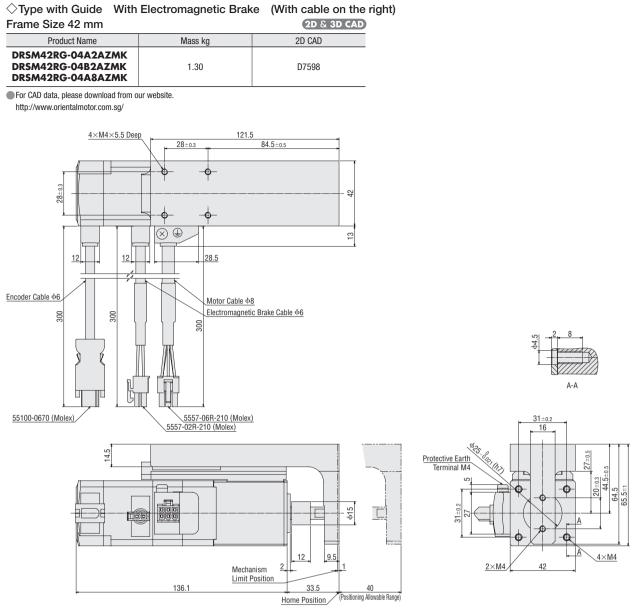
The above figure is an outline drawing of the cable on the right. For outline drawing of the cable on the left, see our website. http://www.orientalmotor.com.sg/
