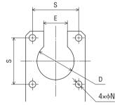
Shape of Actuator Installation Hole
