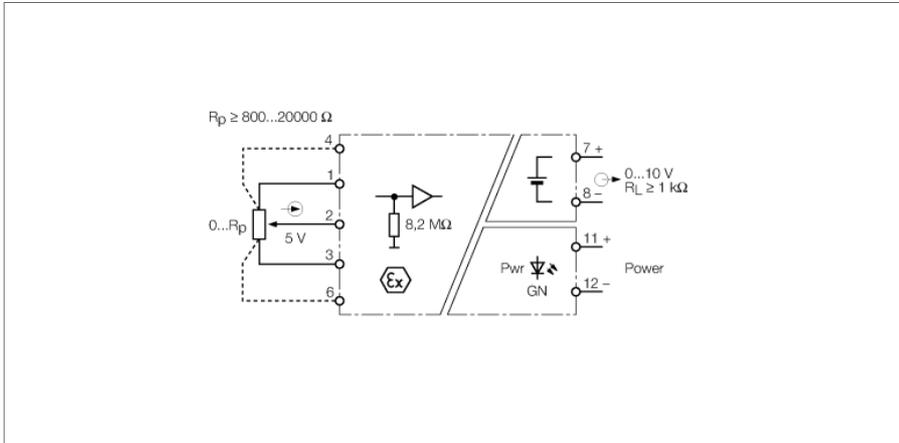
The 1-channel potentiometer amplifier IM36-11EX-U/24VDC is designed to transmit signals from 3 or 5-wire potentiometers galvanically isolated from the Ex area to the non-Ex area and to convert them into normalized 0...10 V analog signals. The resistance value of the wiper contact, ranging from 0 Ω to the nominal resistance value (final value) of the potentiometer, is detected and processed linearly.
